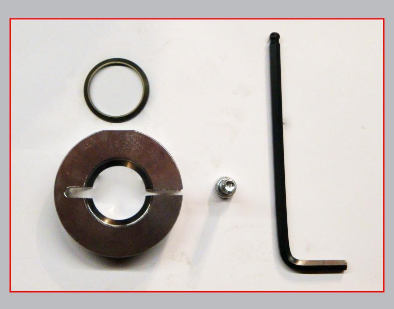
The new CARDI easy release device for bits. Universal use with 1"1/4 UNC standard bits.
