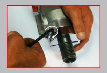
Screw the CARDIFACILE screw with the allen key;
